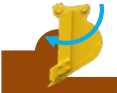
1. Digging (Bucket Curl)
