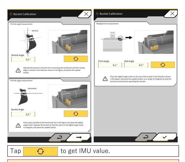
Use a digital angle meter to operate the bucket.
