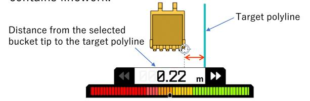
The offset direction depends on the relationship between the position of the bucket and the selected linework.
